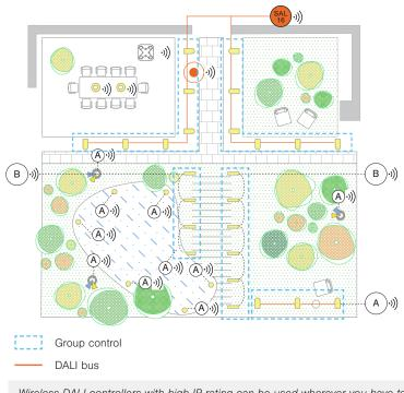
Wireless DALI controllers with high IP rating can be used wherever you have to reckon with moisture during use, for example: Bathrooms, sauna, swimming pools, garden lights, for all outdoor applications.
